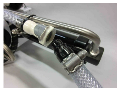
Connecting brine discharge service hose
