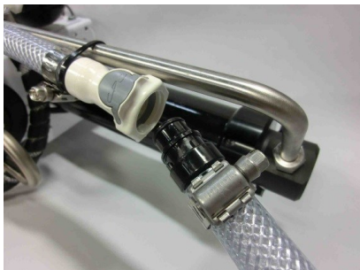
Connecting brine discharge service hose
