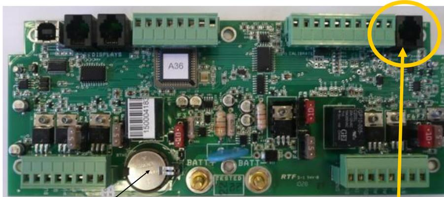
Battery with tab removed
