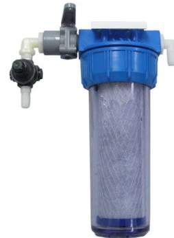
**Boost Pump module:** The boost pump module should be mounted vertically with room to attach the service hose to the outlet on the right side (not visible in photo). The boost pump **MUST** be installed below the waterline to ensure that it will prime. If allowed to run dry it will fail and the feed pump will be damaged.
