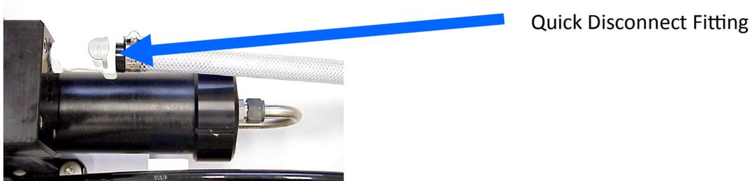
**Fresh Water Flush:** Route a feed line from the domestic cold pressure water system to the 1/2-inch hose barb on the fresh water flush module. This needs to be pressurized when the boat is unattended for the fresh water flush system to function properly. *The domestic fresh water pump must be able to deliver 1.5 gallons per minute (6 LPM) at 25 PSI (1.7 bar).*
