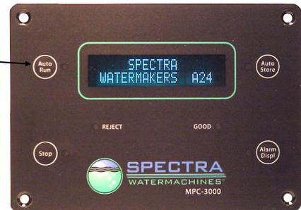
**Single Flush:** Pressing and holding the Auto Store button for 5 seconds will activate the single flush mode:
