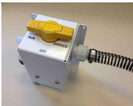
Service hose connected and service valve to SERVICE
