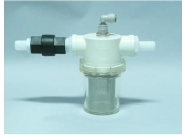
**Flush Cycle Expansion Tank:** This expansion tank maintains water flow during the flush cycle as the feed pump cycles on and off. The feed pump cycles so the flow through the charcoal filter is limited to 1.5 GPH.
