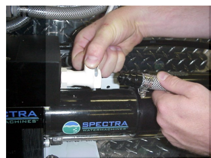
Connecting brine discharge service hose
