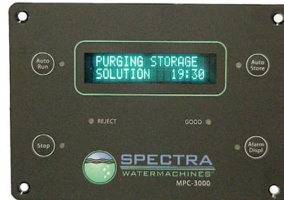
**Note:** If you must stop the purge sequence for any reason, the control will default back to the beginning of the purging mode to protect your system. If you wish, you can bypass the purge sequence and initiate a normal start. Pressing both “Auto Run” and “Stop” simultaneously anytime during the purge sequence will bypass the purge sequence and enable a normal start. In any case **do not pressurize the system for the first twenty minutes** or more.
