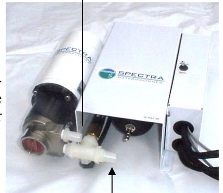
From the inlet thru-hull to the flush module and from the flush module to the pump module inlet use the supplied clear  $\frac{3}{4}$  (19mm) spiral suction rated hose.
