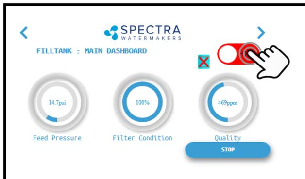
**Note:** The system will automatically drop to Low Mode when it senses high membrane pressure, or low boost (feed) pressure.
