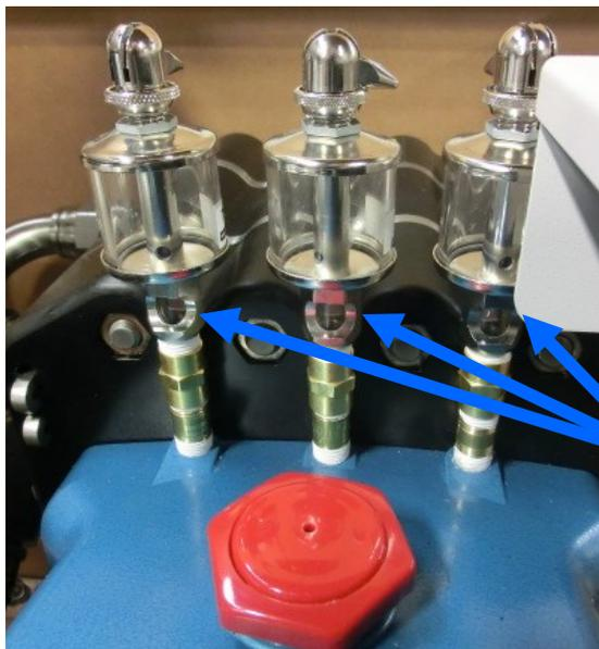
The oilers will drip when opened, which can be seen in the window below the reservoir.
