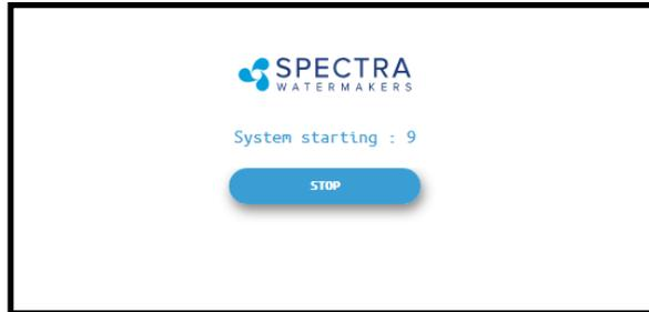
6. Once the Boost Pressure reaches the minimum threshold, the system starts operating and you will be taken directly to the Main Dashboard which shows the current status.
