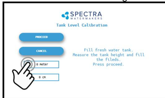
Press the Feet (Meter) field to enter the tank height in feet (meters).
