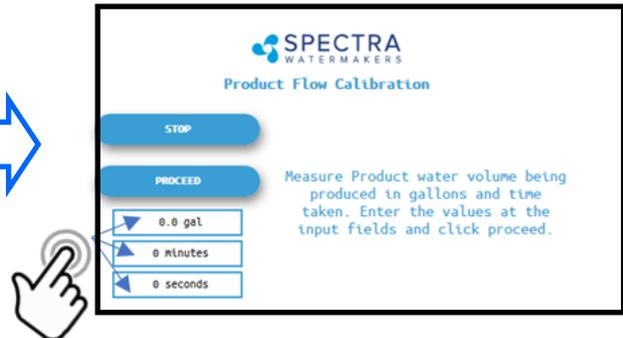
4. Allow the system to run for a few minutes to stabilize and then time in minutes and seconds, how long it takes to fill a container of a known volume.
