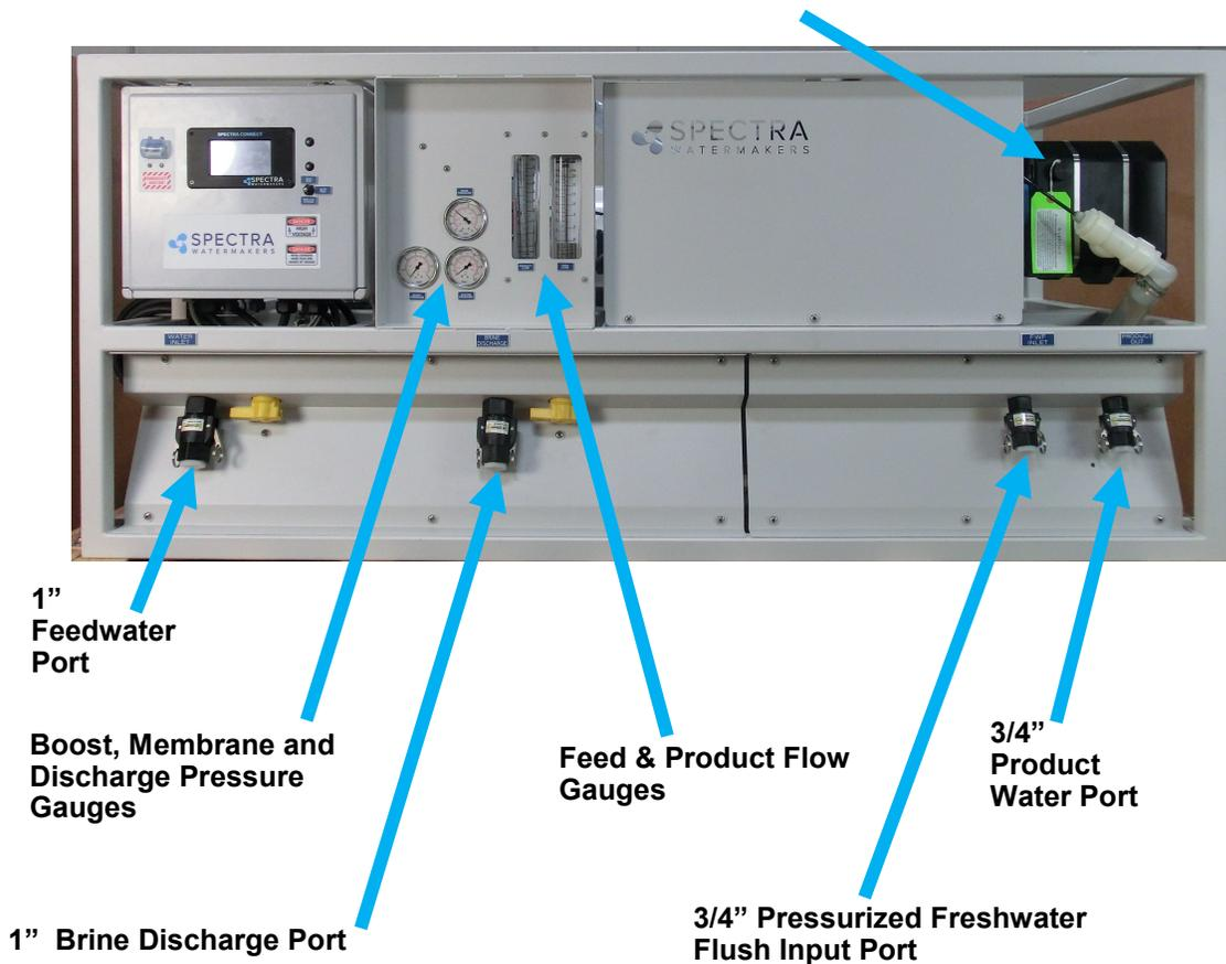
**Note:** The valves for the feed and the brine ports in the photo above are shown in the 'Run' position.
