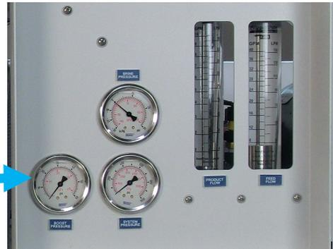
**Note: Boost pressure in excess of 25psi can cause hose failure.**
