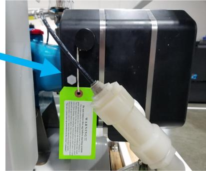
**Technical tip:** Knocking in the Pearson Pump is caused by the boost pressure being either too low or too high. Adjust the boost pressure as high as possible and close the brine discharge valve to add 3-5psi of back pressure.
