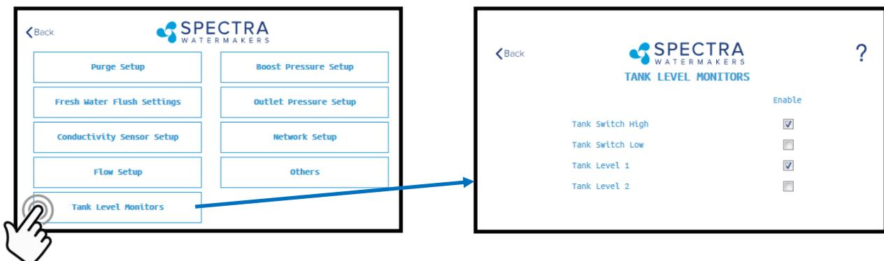
**Tank Setup** - Enable/disable tank sensors.
