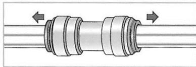
Pull on the tube to check it is secure. Test the system before use.
