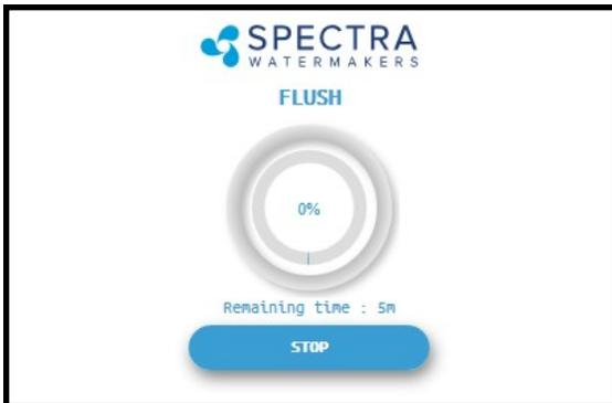
10. After Fresh Water Flushing the system will enter standby mode waiting for the next run cycle.
