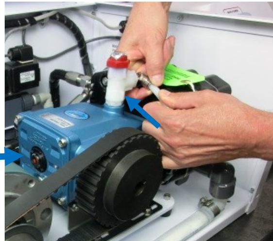
Drain oil into a suitable container.
