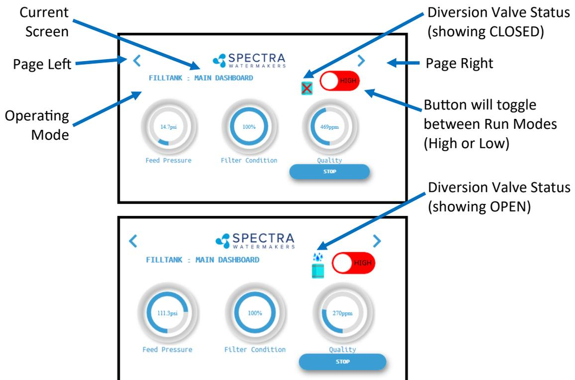
7. When the Product Water Quality is better than the programmed threshold, the Diversion Valve opens, allowing water to enter the tanks and the screen image changes.
