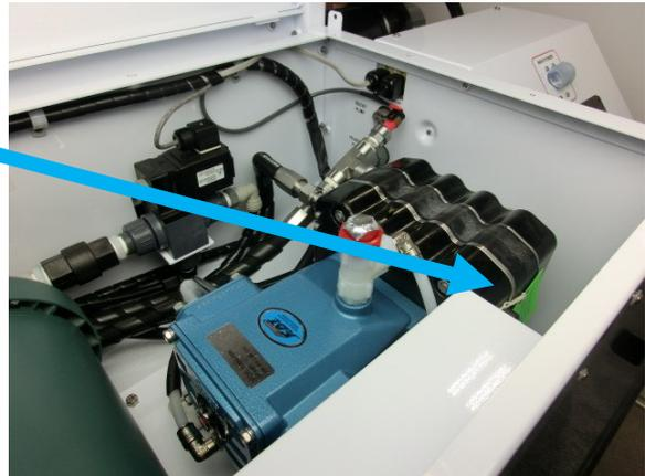
11. The system will now run under pressure and desalinate water. This mode diverts the product water overboard in case there is any residual chemicals in the membrane. Carefully inspect for leaks over the entire system! Shut down the system and repair any leaks you find.
