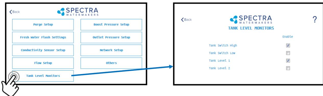
**Tank Setup** - Enable/disable tank sensors.
