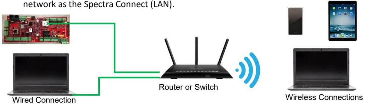
7. On the computer, tablet or smartphone, open a web browser such as Firefox, Chrome, or Safari. In the web address bar at the top, type the 'Device IP' address previously recorded. Press 'Enter'.
