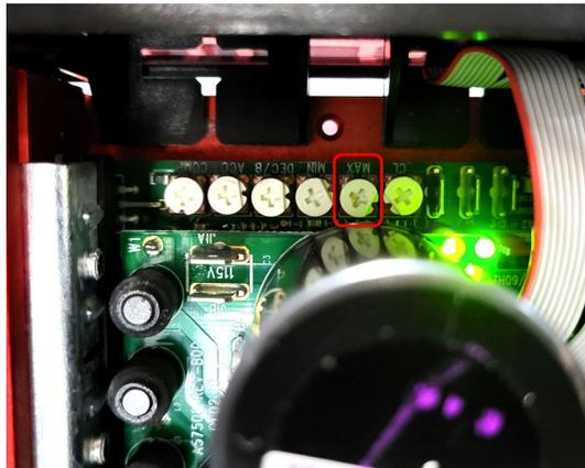
3. You will be adjusting the potentiometer that can be found second from the far right. The potentiometer will read “MAX” labeled upside down. Turn the screwdriver left to slow the Boost Pump speed and reduce the Boost Pressure or turn the screwdriver right to increase Boost Pump Speed.
