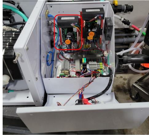
2. You will need a small Phillips head screwdriver to adjust one of the potentiometers on the left VFD (Variable Frequency Drive).
