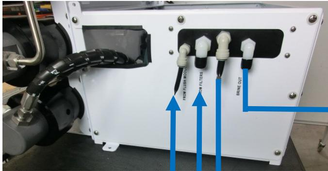
Brine Discharge — Use 5/8" braided hose from the manifold through the Brine Discharge Service Valve and to the thru-hull.
