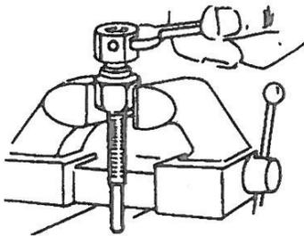
3. When assembling swivel ends, screw threaded mandrel all the way into interior threads of swivel and wrench tight.
