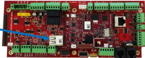
**Note:** If you are connecting directly into a wireless router, **DO NOT CONNECT TO THE WLAN (Wireless Local Area Network)** ethernet port. You must connect to one of the LAN ports typically labeled 1, 2, 3, 4, etc.
