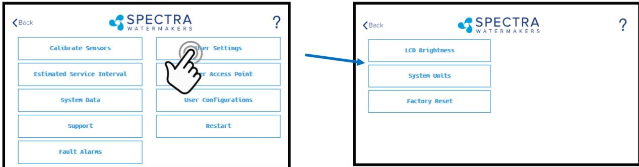
**LCD Brightness:** Set brightness of the hardwired display(s) from 10—100%
