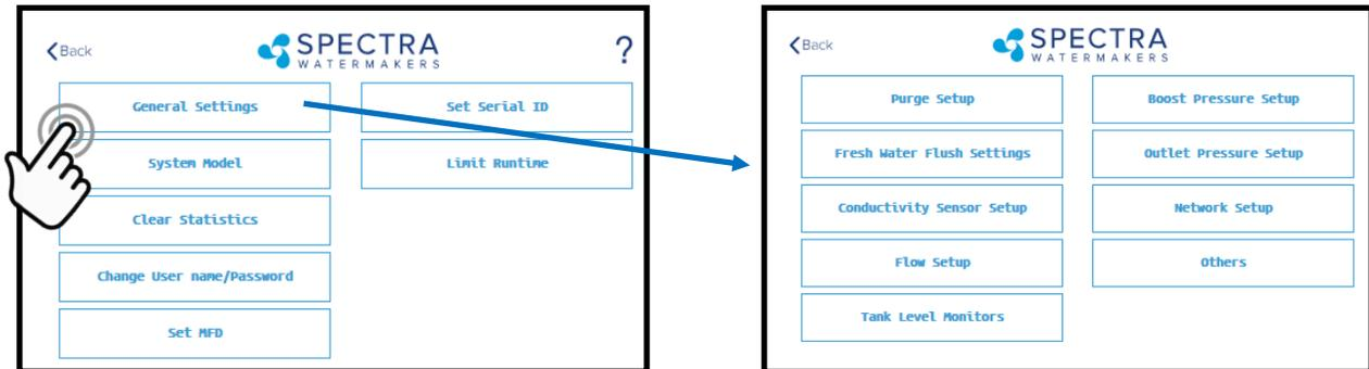
**Purge Setup:** Adjusts the time and maximum feed pressure allowed for the Purge Mode. **CAUTION: Permanent damage to the membrane can occur if this setting is adjusted. Consult the factory before making any adjustments.**
