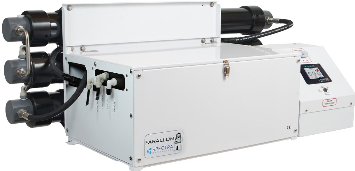
The membrane maximum temperature specification is 113°F (45°C), as specified by the membrane manufacturer. This module must be installed in an area that maintains a temperature below 120°F (50°C). Make sure that the area around and under the pump does not have any water sensitive equipment. Water will be spilled during any repairs or if a leak occurs.
