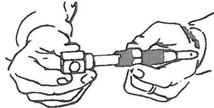
2. When assembling male pipe ends, slide nipple onto mandrel.
