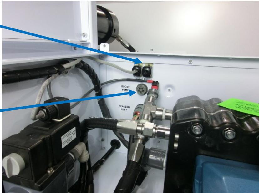
Route the boost pump power cable to the Control Box from the boost pump. Do not get the cable wet, and be careful not to damage the plug or conductors during installation. The boost pump power cable plug is located under the sockets for the Salinity probe and the Remote display. Route the power cable and use cable ties to keep it in place.
