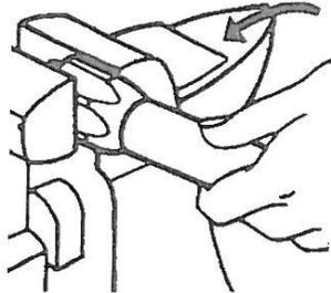
1. Identify Over All Length (OAL) of hose assembly and the Cut Off Allowance (COA) length of fitting(s) on hose ends by use of the fitting data table. Properly measure, mark and cut hose to desired length using fine tooth hacksaw or a cut-off machine. Place socket in vice and screw in hose counter-clockwise until hose bottoms. Back hose out 1/2 turn.
