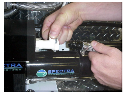
Connecting brine discharge service hose
