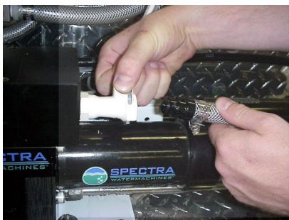
Connecting brine discharge service hose
