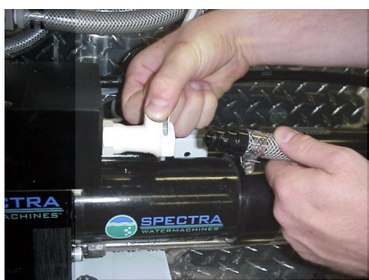
Connecting brine discharge service hose
