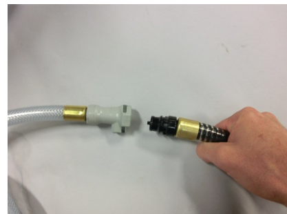
Attaching intake service hose to the hose connecting to the sea strainer.
