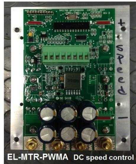
Now when you order a standard Speed Control now each channel will be set to run at 50% of the motors capacity. Each speed will then have to be adjusted with the magnetic reed switches.
