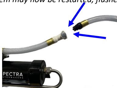
***Connecting brine discharge service hose at quick disconnect
