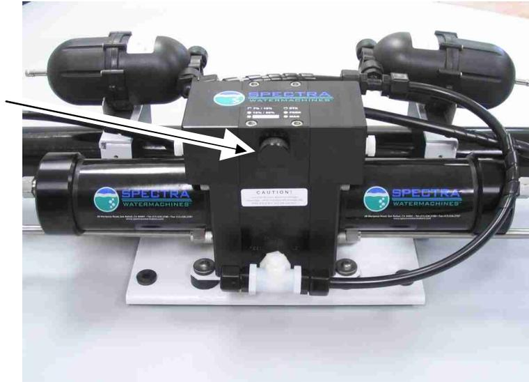
The membrane maximum temperature specification is 120F. This module must be installed in an area that maintains a temperature below 120F (50C). A cool location is preferable. It may be placed as high in the boat as you desire. Make sure that the area around and under the pump does not have any water sensitive equipment. Water will be spilled during any repairs or if a leak occurs.
