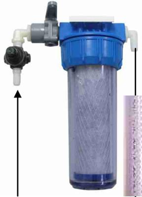
Use the 1/2inch braided hose between the Flush module and the Feed Pump Module
