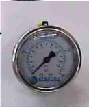
Mount the pressure gauge in the low pressure inlet gauge tee.
