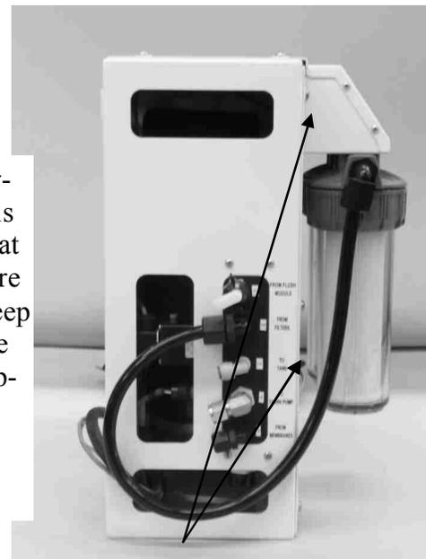
Remove front cover to access mounting holes in the enclosure.
