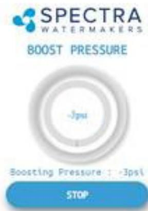
Note: -3 psi is displayed when there is no reading from a pressure sensor.
