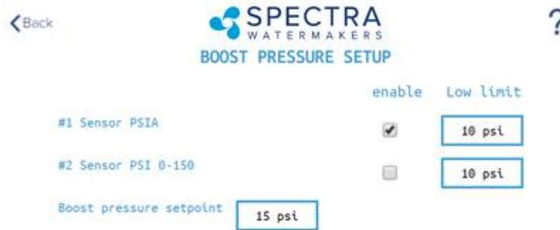
The factory default for the Boost Pressure Set Point is 15 psi. This value was chosen because it is just above atmospheric pressure of 14.7 psi. Once the inlet of the pump reaches atmospheric pressure the feed pump is no longer running in a vacuum. Once the Boost Pressure Set Point is reached the feed pump turns on and the run cycle begins its next phase.
