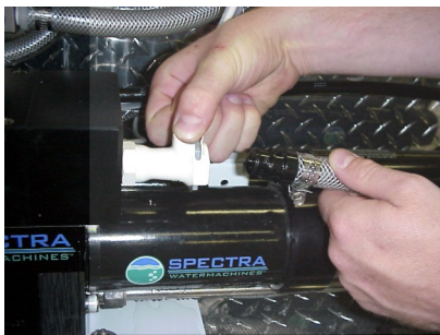
Connecting brine discharge service hose
