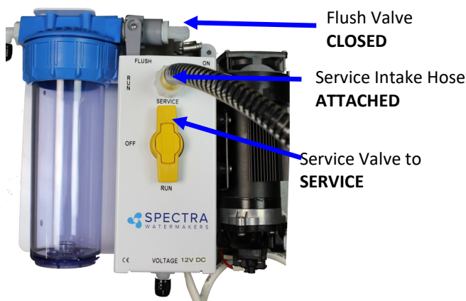
Valves in SERVICE position:
