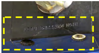
Example of a crack due to over tightening.
