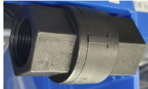
This one way valve is used in the intake path to ensure seawater can only flow one direction. Old documentation mistakenly listed this as a Clark Pump part.
