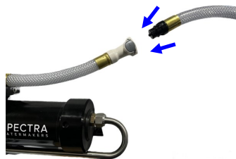
*Connecting brine discharge service hose at quick disconnect
