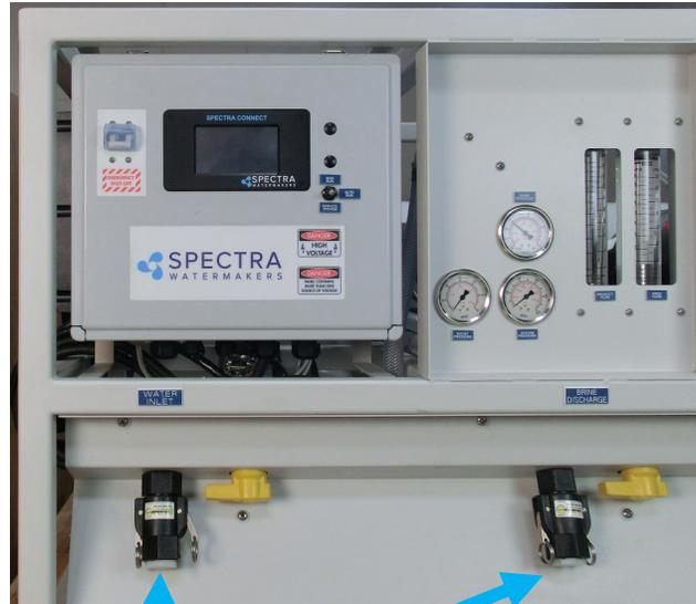
Attach the service hoses, place the open ends of the hoses in the bucket and turn both the service valves to SERVICE (valves in picture shown in run position)
