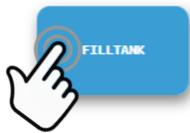
3. Runs your watermaker until the Tank Full switch closes, fresh water flushes the system, then goes into 'Auto Store' mode and the Flush Interval timer starts. *This is the default mode of operation.*
