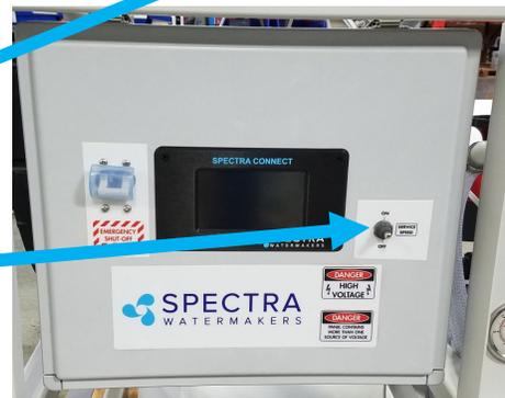
Circulate cleaning chemicals for up to 6 hours depending on the level of fouling present (contact Tech Support for advise on cleaning).
