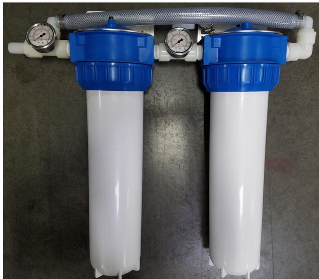
**Note:** Filter housings should always be tightened by hand, do not use the wrench. Overtightening the collar will not improve sealing. If the housing leaks when hand tightened then the O-ring needs to be cleaned and greased (silicone grease only). A small amount of silicone grease on the threads will make it easier to remove the collar.
