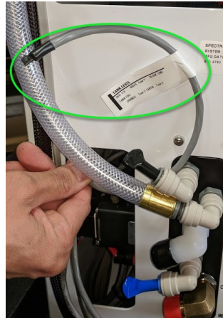
5 Conductor wire: Tank Full Switch, Green + Orange
