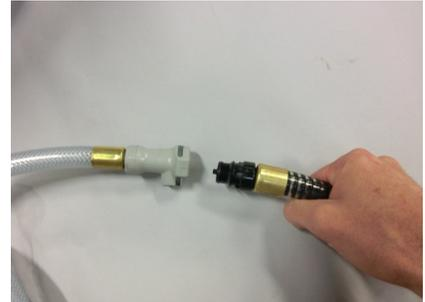
Attaching intake service hose to the hose connecting to the sea strainer.
