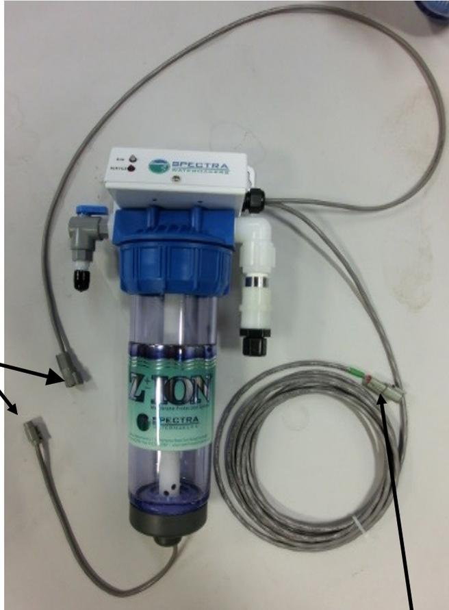
Plugs into green pigtail on right side (opposite side from the manifold) of the feed pump module.
