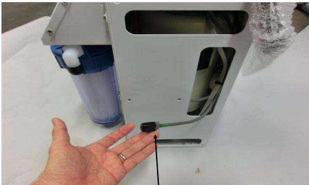
Z-ION Connector (with black protective cover) on feed pump module.
