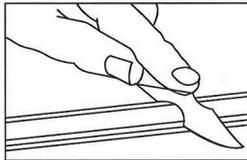
Cut the tube squarely and remove any burrs.
