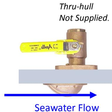
**Thru-hull Type and Location:** The system must be connected to a dedicated 3/4" to 1" forward-facing scoop-type intake thru-hull and seacock.
