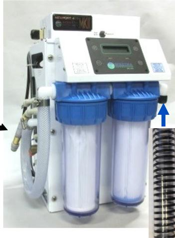
Feed water inlet from boost pump. Leave enough extra length in this hose to allow the front cover to be moved aside for service access to the inside of the box.
