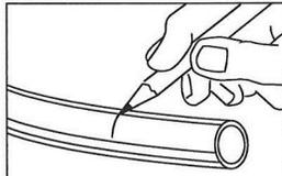
Mark from end of tube the length of insertion. (See table below)
