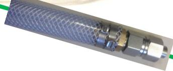
Use the 1/2-inch braided vinyl hose, pre-fitted on one end with a hose-to-high pressure adapter to connect to fitting on feed pump manifold labeled "To Clark Pump." The other end is fitted with a John Guest stem adapter, which will plug into one side of the John Guest tee on the feed water inlet of the Clark Pump. (Remove plug first. See page 22 for John Guest fitting instructions.)
