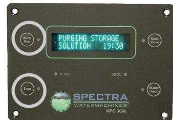
5. After the purge sequence the display will alarm with the message **“Close pressure relief valve.”** **Close the valve** and proceed by pressing **Auto Run** again. **If the system has been stored with propylene glycol, purge the system for 4-6 hours WITH THE PRESSURE RELIEF VALVE OPEN by flipping the toggle switch to the RUN MANUAL position.**
