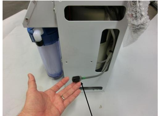
Z-ION Connector (with black protective cover). Left unused if your system was not ordered with the optional Z-ION.
