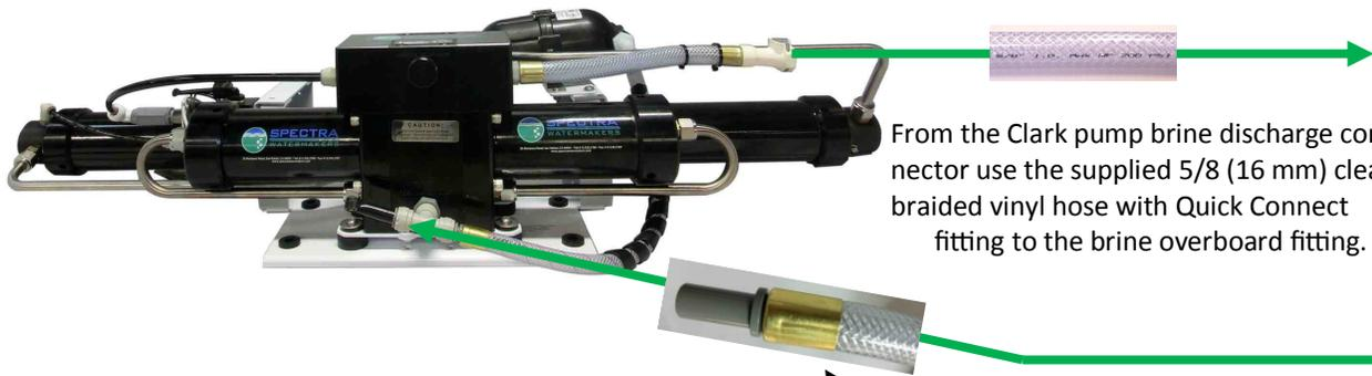
From the Clark pump brine discharge connector use the supplied 5/8 (16 mm) clear braided vinyl hose with Quick Connect fitting to the brine overboard fitting.
