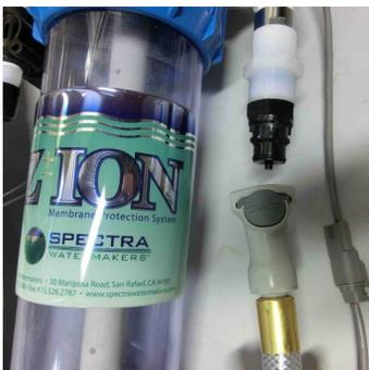
Attaching 1/2-inch vinyl hose to sea strainer using the 3/8" John Guest stem fitting and hose clamp found in installation kit:
