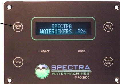
**Auto Store:** Pressing the Auto Store button, in the top right corner of the display, will activate the automated storage sequence. This will automatically store the system, performing a fresh water flush once every 1 - 30 days, according to the flush timer interval settings programmed into the MPC:
