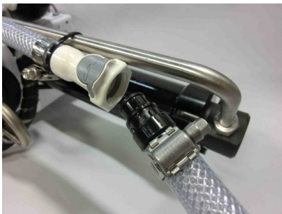
Connecting brine discharge service hose
