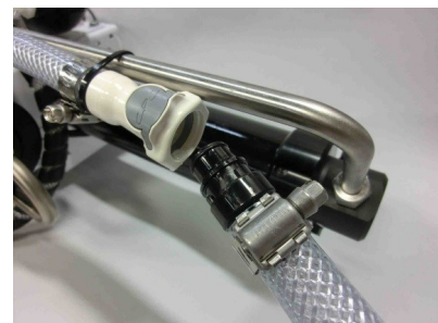
Connecting brine discharge service hose
