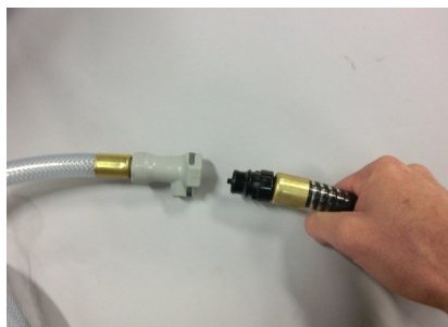
Attaching intake service hose to hose to sea strainer.
