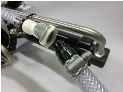
Connecting brine discharge service hose
