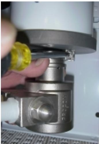
Loosen the V band clamp until the pump head can be removed. The suction and inlet hoses will come out with it. Remove the green bonding wire from the stud on the pump body.
