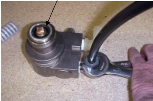
Using two wrenches, loosen the compression nut on the high pressure discharge fitting. Remove and set aside the hose
