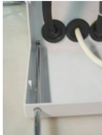
A long screwdriver will be required to access the fasteners
