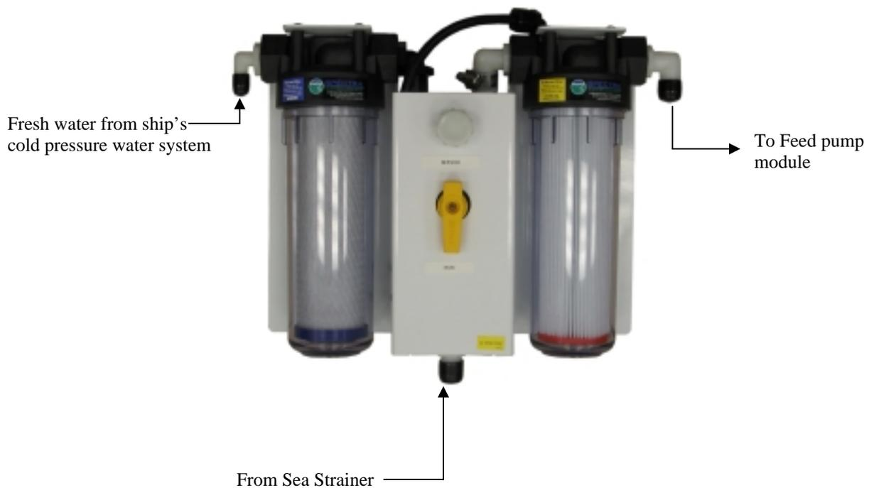
From the inlet thru hull to the flush module and from flush module to the pump module inlet use the supplied clear 3/4 (19mm) spiral suction rated hose. The outlet of the filter assembly on the main module to the Clark pump assembly is under a pressure of 200 PSI (14.5 bar). Use the supplied 1/2" (12.7mm) tubing. Follow the HP tube assembly instructions (p.47). From the Clark pump brine discharge quick disconnect fitting use the supplied 5/8 (15.9mm) clear braided vinyl hose.
