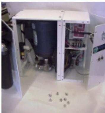
Remove front covers to access mounting holes in the enclosure.
