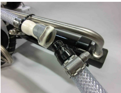
Connecting brine discharge service hose
