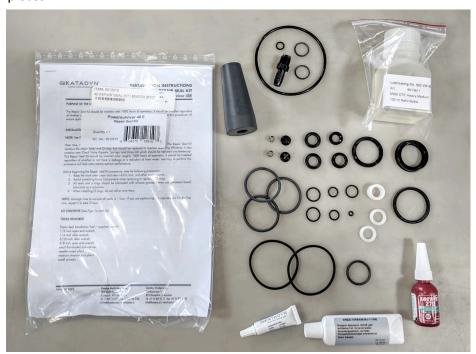
• The Spool Valve Kit (8016525) comes with the unit and is a highly recommended spare. After a bucket test, it is the first suggestion when water moves through the system easily, but no product water is being made.
