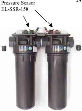
There are two pressure sensors and a vacuum sensor on MPC-3000 and MPC-5000 Mk I automated units.
