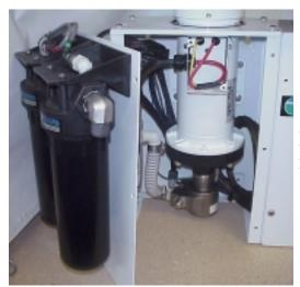
Remove the front cover of the pump control module. Leave filters attached.
