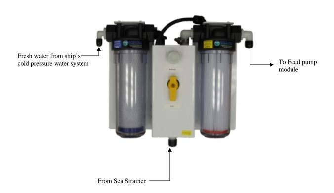
From the inlet thru hull to the flush module and from flush module to the pump module inlet use the supplied clear 3/4 (19mm) spiral suction rated hose. The outlet of the filter assembly on the main module to the Clark pump assembly is under a pressure of 200 PSI (14.5 bar). Use the supplied 1/2" (12.7mm) tubing. Follow the HP tube assembly instructions (p.47). From the Clark pump brine discharge quick disconnect fitting use the supplied 5/8 (15.9mm) clear braided vinyl hose.
