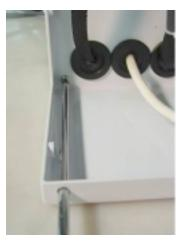
A long screwdriver will be required to access the fasteners
