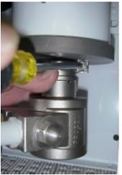
Loosen the V band clamp until the pump head can be removed. The suction and inlet hoses will come out with it. Remove the green bonding wire from the stud on the pump body. Loosen the hose clamp on the inlet hose and remove the hose from the fitting.
