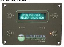
Push the **Auto Run** Button. The feed pump will start and the message "**Purging Storage Solution**" will appear:
