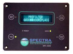
The MPC 5000 board is fully programmable from the remote display. Instructions on how to access and adjust the operating parameters are on page 76 of this manual.
