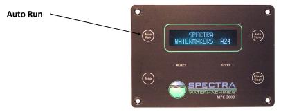
**Auto Store:** Pressing the Auto Store button, in the top right corner of the display, will activate the automated storage sequence. This will automatically store the system, performing a fresh water flush once every 1 - 30 days, according to the flush timer interval settings programmed into the MPC:
