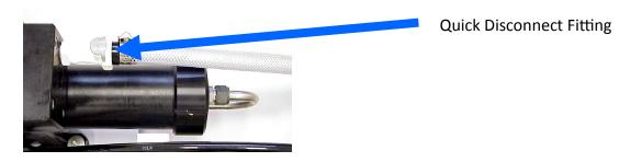
Fresh Water Flush: Route a feed line from the domestic cold pressure water system to the 1/2-inch hose barb on the fresh water flush module. This needs to be pressurized when the boat is unattended for the fresh water flush system to function properly. The domestic fresh water pump must be able to deliver 1.5 gallons per minute (6 LPM) at 25 PSI (1.7 bar).
