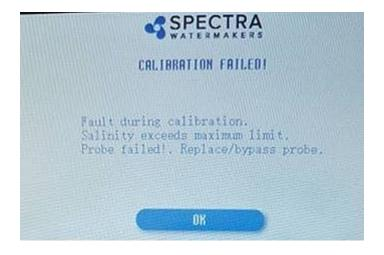
Many times, this can be resolved by running the watermaker for a short time until the salinity reading is within range, at which point calibration can be attempted again.
