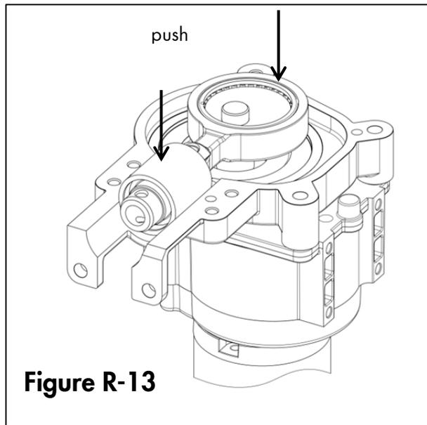
Lubricate the needles of the needle bearing with grease.
