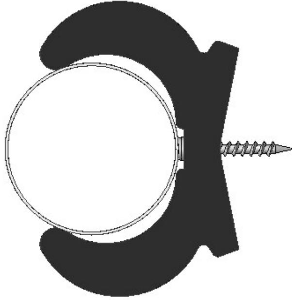
2. HOUSING MOUNT WITH MEMBRANE HOUSING IN PLACE.
