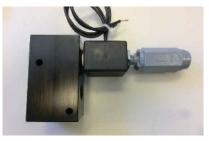
To replace a failed solenoid valve on an older system we have created an adapter (part number PL-MNF-ECI-SPAR) to fit a Spartan valve to an older-style manifold. To seal properly, the adapter must have a Spartan 4mm orifice insert (part number SLN-SPA4MOR) and an adapter O-ring (part number SO-MNF-SP/ECIAD).
