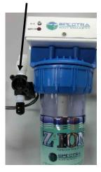
Unfortunately Alcon has stopped manufacturing these solenoid valves, so we have found a substitute made by Spartan Scientific. The Spartan valves have the same sized orifices as the Alcon valves, so they won't alter the water flow, but Spartan valves have smaller threaded bases, and the output fitting on the Spartan diversion valve is smaller (1/8-inch NPT instead of 1/4-inch NPT):
