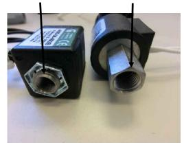
On new systems we will mill the receptacle for the smaller bases on the Spartan valves into the manifolds, so the change will be seamless. You will start to see the Spartan valves on new systems as we make the change over the next few months.
