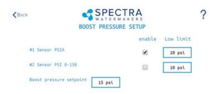
The factory default for the Boost Pressure Set Point is 15 psi. This value was chosen because it is just above atmospheric pressure of 14.7 psi. Once the inlet of the pump reaches atmospheric pressure the feed pump is no longer running in a vacuum. Once the Boost Pressure Set Point is reached the feed pump turns on and the run cycle begins its next phase.
