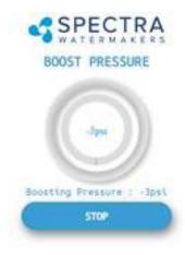
Note: -3 psi is displayed when there is no reading from a pressure sensor.
