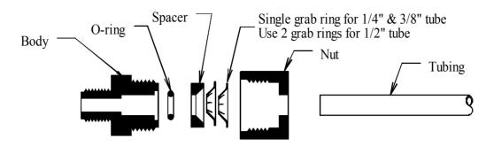
Step 1: Dissemble fitting components
