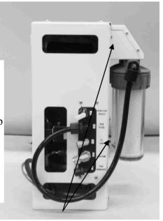
Remove front cover to access mounting holes in the enclosure.
