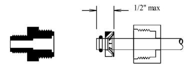
Step 2: Install the Nut first then use the bevelled side of the Spacer to push the Grab Ring onto the tube no more than 1/2". Slip the O-ring over the tube to hold the Spacer in place. If the Grab Ring is pushed too far, trim back the tube so about 1/4" of tube extends past the O-ring.
