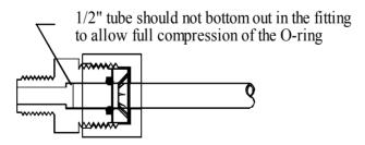
Step 4: Hand tighten the nut. DO NOT OVER TIGHTEN! DO NOT USE A WRENCH! The tube should not come out if pulled by hand. If it does, tighten the grab ring tabs.
