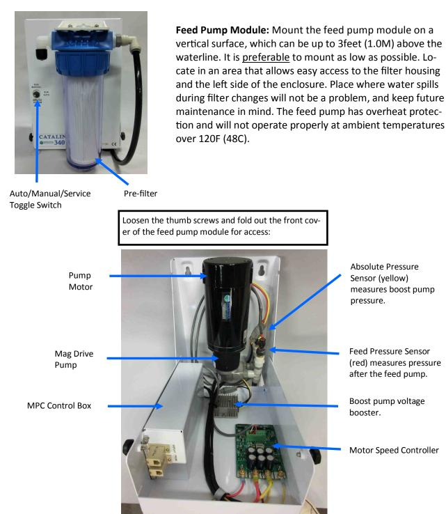
**Note:** When plumbing the Catalina feed pump module, route the feed water hose so that the front cover may be opened without removing the hose or tubing. All tubing connections are made using John Guest connectors, shown on page 22. After assembling all plumbing fittings, thoroughly check for leaks.
