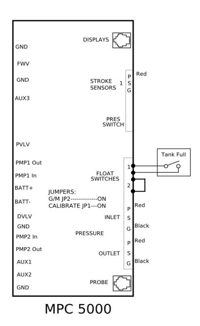
Tank Switch Wiring: Tank full switch wired to Float Switch 1 terminals; jumper across Float Switch 2 terminals
