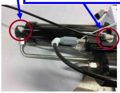
3. Connect the tube from the tank directly to the membrane/ pressure vessel.
