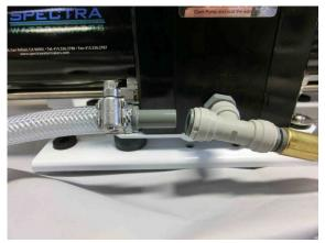
**Brine Discharge:** Route the brine discharge from the quick disconnect fittings to a thru-hull above the waterline using the supplied 5/8" braided vinyl hose and the male Quick Disconnect fitting from the installation kit:
