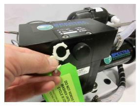
Power up the system by turning on the circuit breaker. After a few seconds a message on the display will read "**Open Pres**sure Relief Valve Now":
