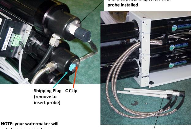
C-Clip and retaining screw with
