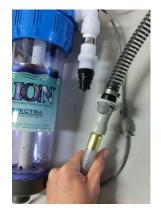
Replacing fresh water flush hose with intake service hose
