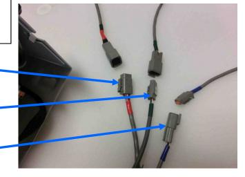
50' (15M) cable with connectors for the MPC-5000 control display
