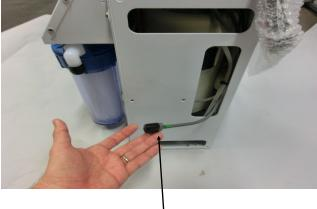
Z-ION Connector (with black protective cover) on feed pump module.
