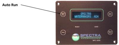
**Auto Store:** Pressing the Auto Store button, in the top right corner of the display, will activate the automated storage sequence. This will automatically store the system, performing a fresh water flush once every 1-30 days, according to the flush timer interval settings programmed into the MPC:
