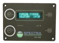
5. After the purge sequence the display will alarm with the message "Close pressure relief valve." **Close the valve** and proceed by pressing **Auto Run** again. **If the system has been stored with propylene glycol, purge the system for 4-6 hours WITH THE PRESSURE RELIEF VALVE OPEN by flipping the toggle switch to the RUN MANUAL position.**
