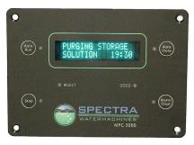
**Note:** If you must stop the purge sequence for any reason, the control will default back to the beginning of the purging mode to protect your system. If you wish, you can bypass the purge sequence and initiate a normal start. Pressing both "Auto Run" and "Stop" simultaneously anytime during the purge sequence will bypass the purge sequence and enable a normal start. In any case **do not pressurize the system for the first twenty minutes** or more.
