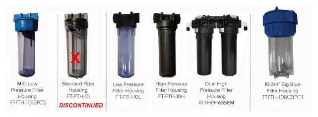
If looking for FT-FTH-10, replacement depends on whether low pressure or high pressure housing is needed. If feed pump is located PRIOR to prefilters, use high pressure. If feed pump is located AFTER prefilters, use low pressure.
